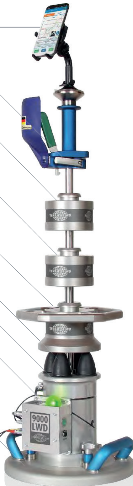
Load plate „DUO-SWITCH“ to change the load plate diameter 300/150 mm resp. 11.8"/5.9". 100 mm/3.9" load plate included.
